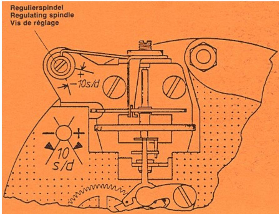
Showing the regulator for adjusting the timekeeping. The screw at the very top left is turned with a screwdriver. Make only a small adjustment each time (about 1/16 of a turn).
